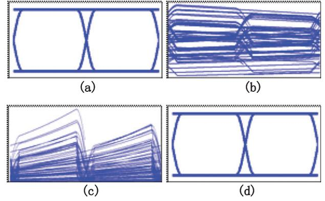
**Figure 1.** (a) The eye diagram of a  $10 \text{ Gb s}^{-1}$  NRZ-OOK signal, (b) the encrypted  $10 \text{ Gb s}^{-1}$  signal by a 500 MHz-spaced 3-line SBS gain, (c) the encrypted  $10 \text{ Gb s}^{-1}$  signal by a 500 MHz-spaced 3-line SBS loss, (d) the decrypted  $10 \text{ Gb s}^{-1}$  signal.
