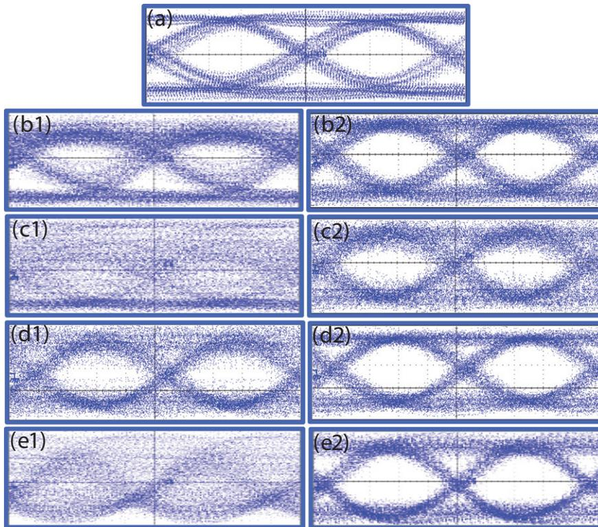
**Figure 4.** The eye diagrams of the original signal (a), the encrypted signals by 2 dB SBS gain (b1), 4 dB SBS gain (c1), 5 dB SBS loss (d1), 10 dB SBS loss (e1) and the decrypted signals by 2 dB SBS loss (b2), 4 dB SBS loss (c2), 5 dB SBS gain (d2), 10 dB SBS gain (e2).
